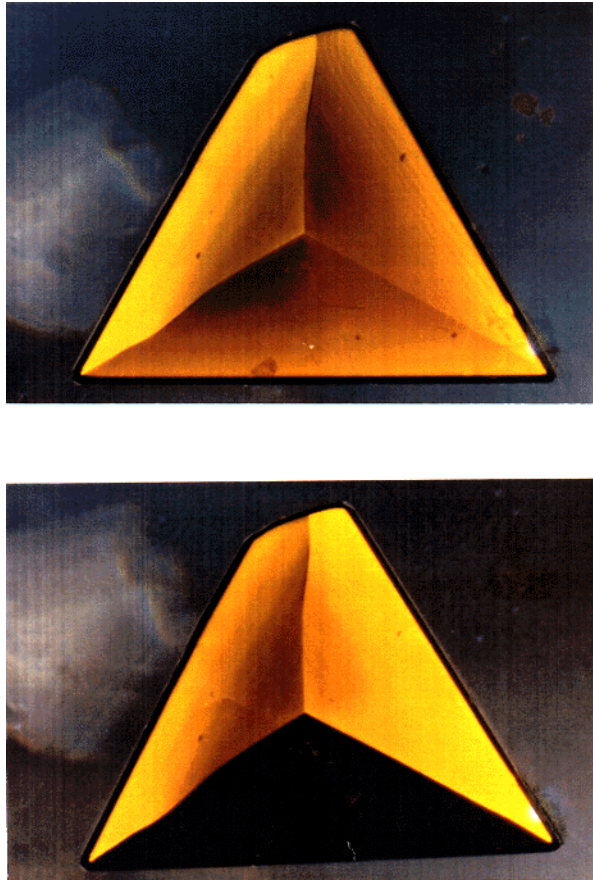
Figure 1. Crystal CRY(111) under crossed polarizers. At the bottom, one of the three sectors is in extinction. Sectors can be successively brought into extinction by rotation of 120^\circ .
